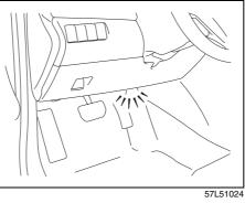
A footwell light is provided in the leg space in front of each front seat. When a front door is opened, the footwell light on the same side lights automatically.
